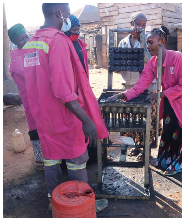
Members of the Kyosimba Onany Saving group demonstrate how to make briquettes, Bwaise III Parish, Kampala, Uganda, F Kizza, 2023
